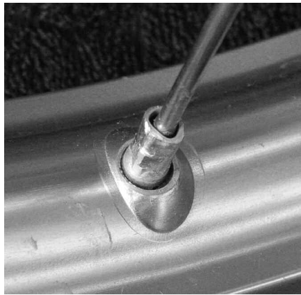
Left: A perfect fit between spoke wrench and nipple makes the job easy and... (Center) prevents this from happening. Not only is this nipple rounded, it's also become crushed against the spoke threads, making it doubly difficult to remove. Right: Once loosened "topside" with a wrench, nipples can be unscrewed easily from the other side.
