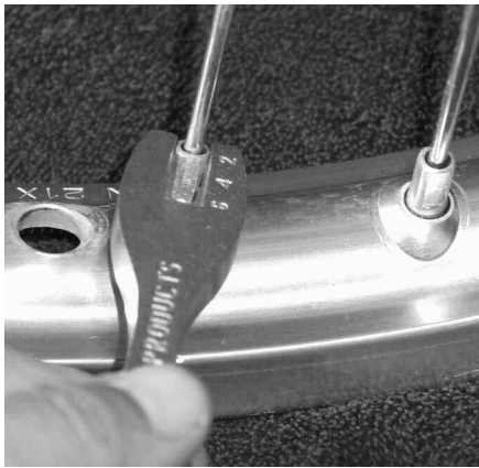
Left: A perfect fit between spoke wrench and nipple makes the job easy and... (Center) prevents this from happening. Not only is this nipple rounded, it's also become crushed against the spoke threads, making it doubly difficult to remove. Right: Once loosened "topside" with a wrench, nipples can be unscrewed easily from the other side.
