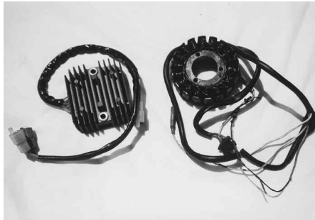
A two-piece system, this one from the infamous early Suzuki GS-series—nicely toasted.
