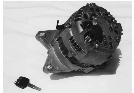
The air-cooled one-piece alternator with its regulator/rectifier inside—much more durable.
